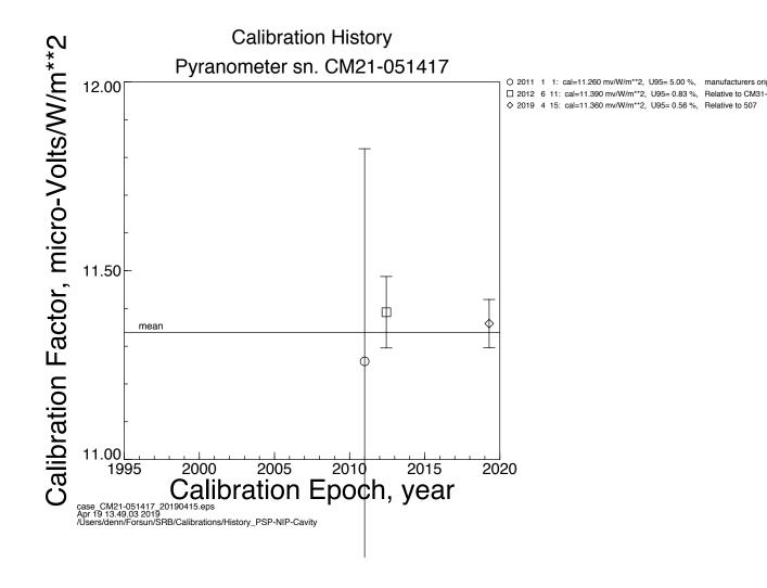
Calibration history for pyranometer CM21-051417. The solid horizontal line represents the mean value. The symbols and their error bars represent the mean and U95 of each calibration event. The column on the right presents numerical values for each calibration event and a brief description of the calibration method used.
