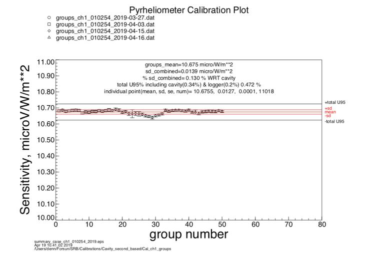
Calibration coefficients for several days. Each symbol represents a cavity run which is approximately 25 minutes. These data are combined to get a final calibration coefficient for the entire, multi-day, calibration session.
