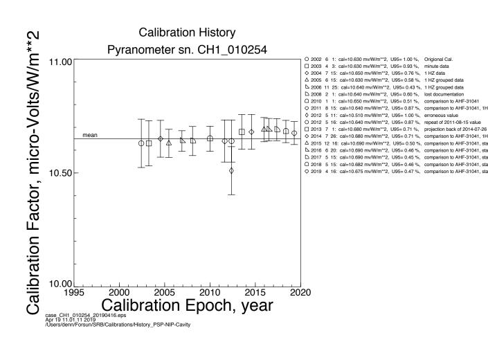
Calibration history for pyrheliometer CH1-010254. The solid horizontal line represents the mean value. The symbols and their error bars represent the mean and U95 of each calibration event. The column on the right presents numerical values for each calibration event and a brief description of the calibration method used.
