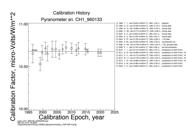
Calibration history for pyrheliometer CH1-960133. The solid horizontal line represents the mean value. The symbols and their error bars represent the mean and U95 of each calibration event. The column on the right presents numerical values for each calibration event and a brief description of the calibration method used.
