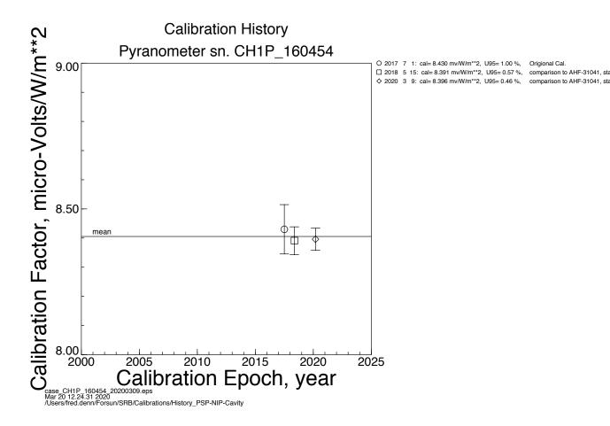
Calibration history for pyrheliometer CHP1-160454. The solid horizontal line represents the mean value. The symbols and their error bars represent the mean and U95 of each calibration event. The column on the right presents numerical values for each calibration event and a brief description of the calibration method used.
