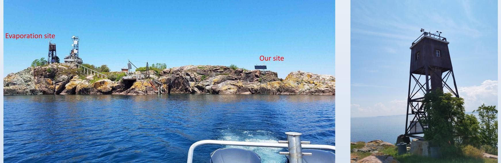
Left: ~ 75 meters is the distance between our measurement site and the eddy covariance/evaporation measurement site. Middle: The bell tower. Right: Eddy covariance/evaporation instrumentation on top of the bell tower. NASA Langley is interested in combining measurements from these two sites along with CERES satellite data to improve understanding of Earth's energy budget.
