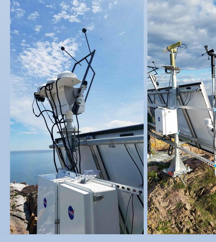
Left: Kipp and Zonen (K&Z) Solar Tracker with K&Z direct, diffuse, global and longwave instrumentation. Right: AERONET sunphotometer and meteorological instruments. Communications are by way of serial over IP and Freewave radios. All instrumentation and almost all hardware are rated to endure the frigid winters.
