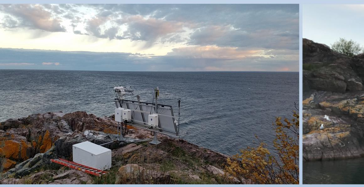
Left: Full view of the entire installation. The large white box is the battery enclosure housing eighteen batteries wired in series and parallel for a 12 volt powered system. Right: View from boat. Our site is approximate 10 m above the water line. Four solar panels regulated by two charge controllers charge the batteries.
