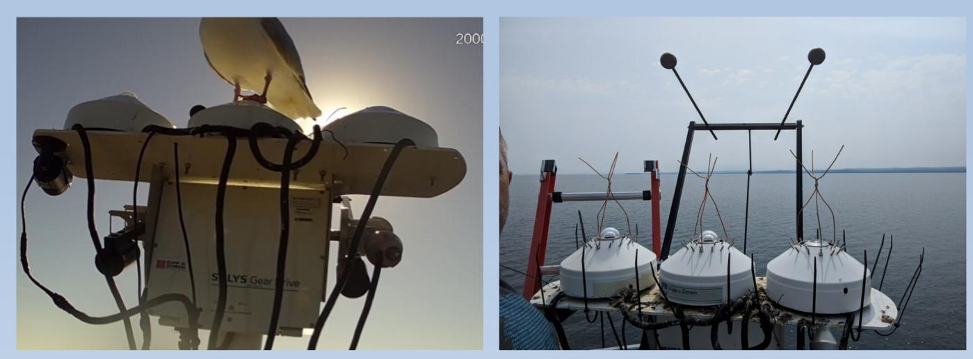
Left: Seagulls were found to be perching on the instruments soon after they were installed. Right: The solution to the seagull problem was modifying the shields with inverted screws and wire. After installation of the new shields, no seagulls have been seen perched on the instruments.
